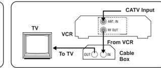
With this connection, you can view one scrambled cable channel while recording another unscrambled channel.
